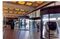
*The Personal Rapid Transport (PRT) system has 10 passenger and 3 freight vehicles serving 2 passenger and 3 freight stations connected by approximately one mile of track. The system is in operation 18 hours a day, 7 days a week serving the Masdar Institute.*
